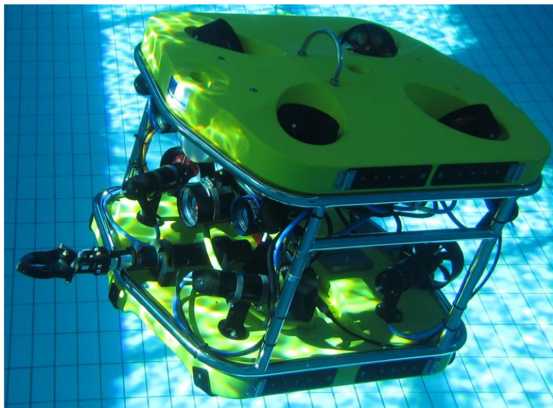
Figure 2. Ocean Modules ROV M500 with mobility in 6 degrees of freedom.
