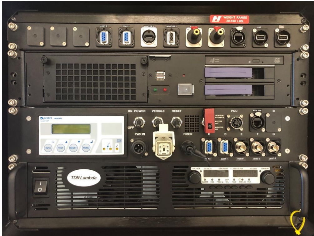
Figure 8. Surface Unit consisting of: Surface Expansion Unit, Computer, Surface Interface Unit and the Power Unit.
